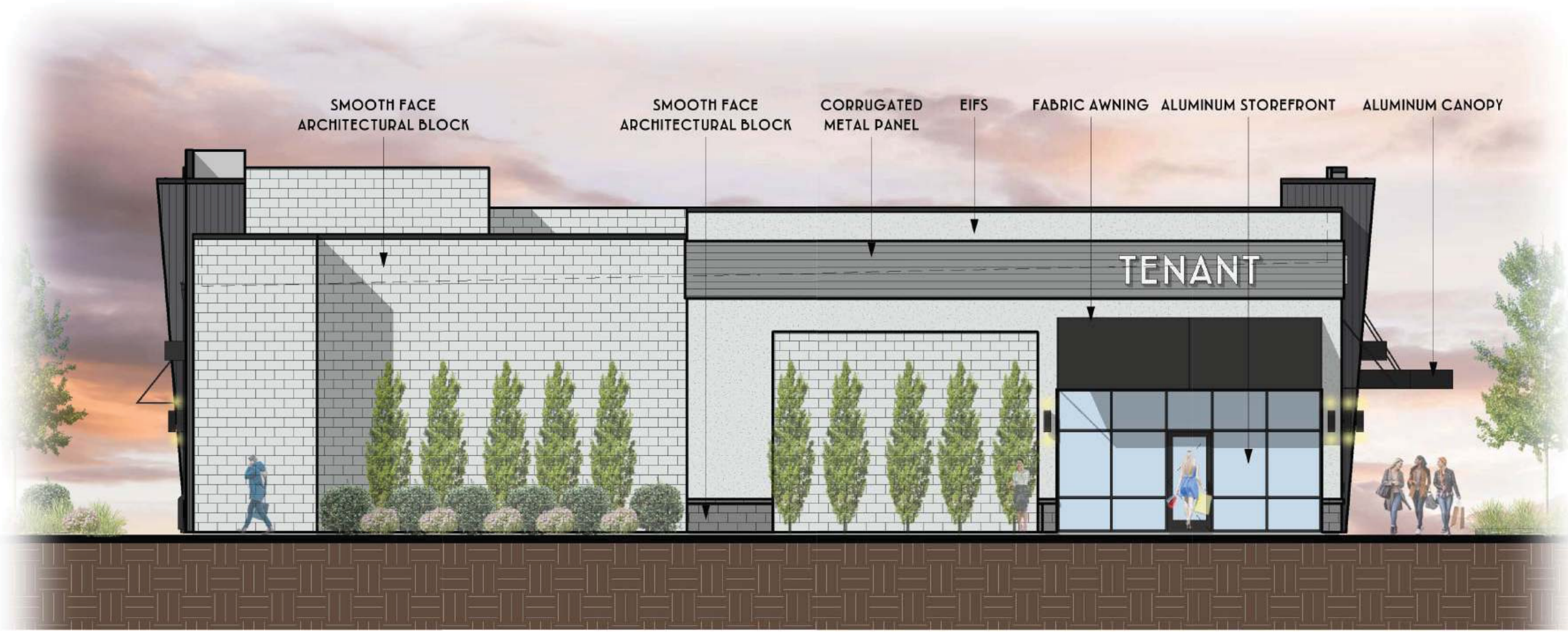
2 LEFT SIDE ELEVATION - NORTHWEST A4-2.1 1/8" = 1'-0"
