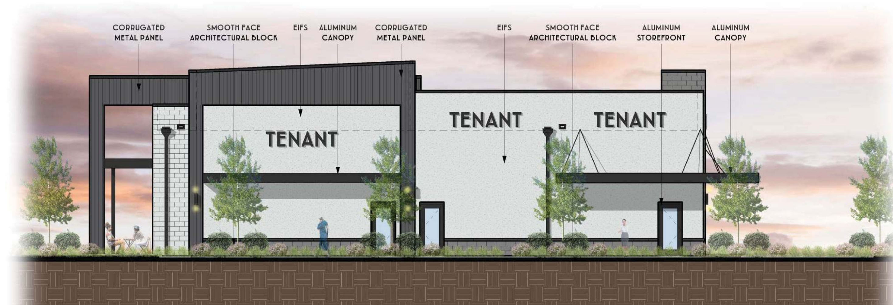
4 REAR ELEVATION - SOUTHEAST A4-7.1 1/8" = 1'-0"
