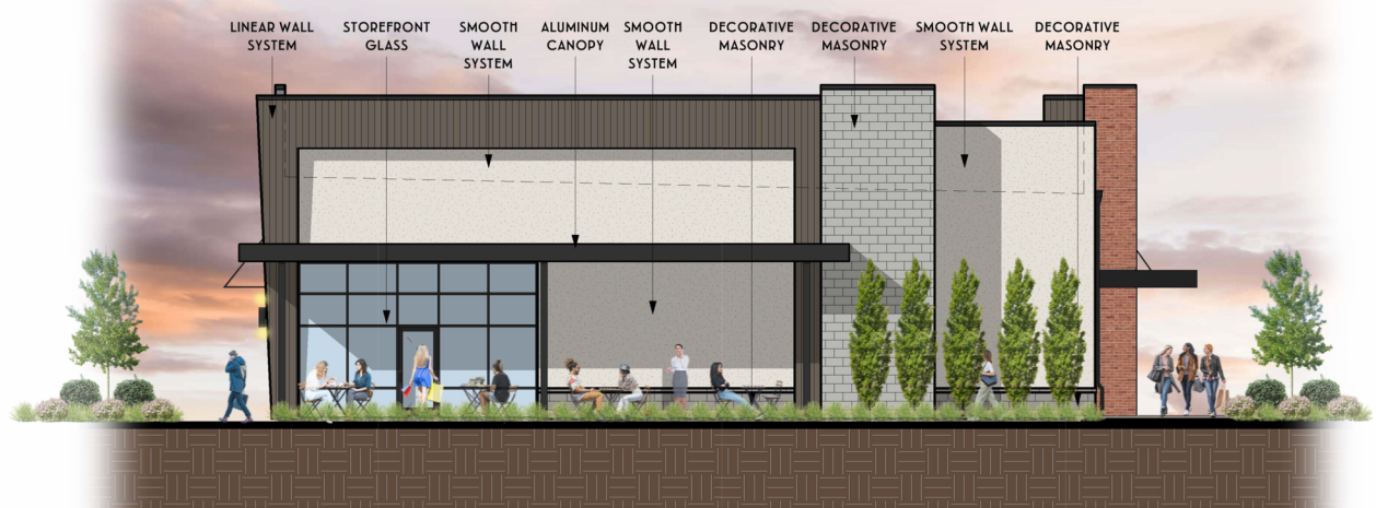
3 RIGHT SIDE ELEVATION - NORTHWEST A4-6.1 1/16" = 1'-0"
