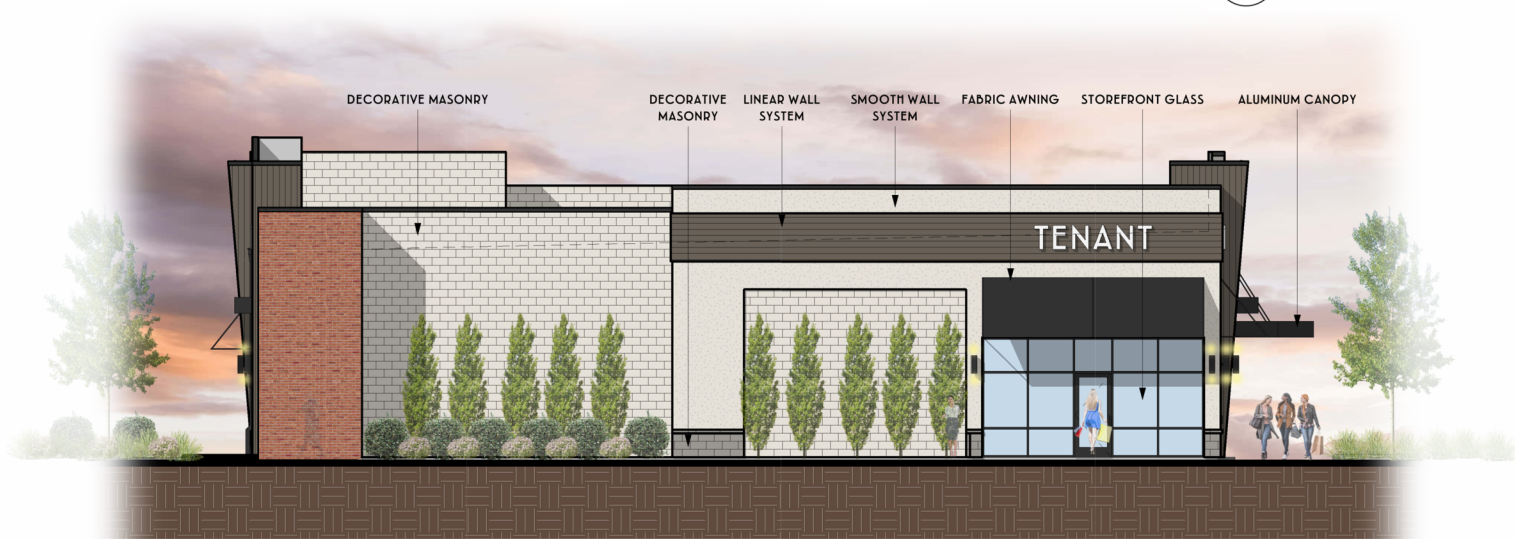
2 LEFT SIDE ELEVATION - NORTHWEST A4-2.1 1/16" = 1'-0"
