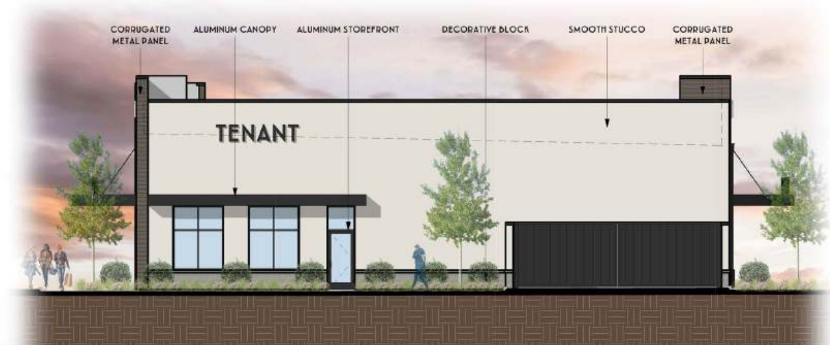
3 RIGHT SIDE ELEVATION - SOUTHEAST A4-4.1 1/16" = 1'-0"
