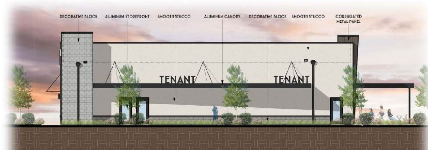
4 REAR ELEVATION - NORTHWEST A4-5.1 1/16" = 1'-0"
