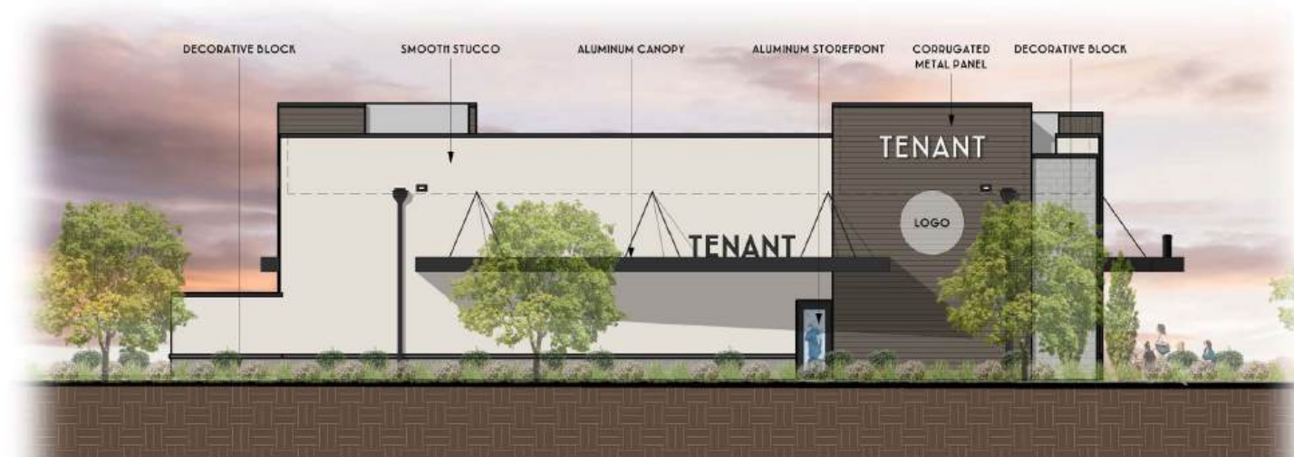
4 REAR ELEVATION - NORTHEAST A4-4.1 1/16" = 1'-0"
