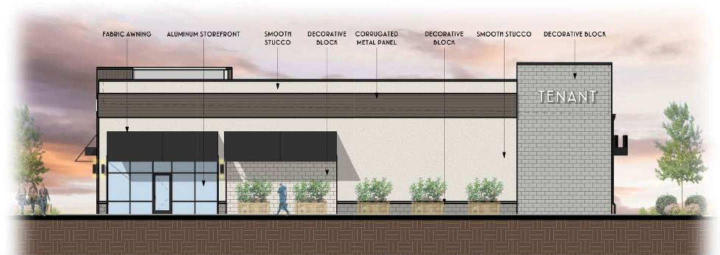
3 RIGHT SIDE ELEVATION - NORTHEAST A4-5.1 1/16" = 1'-0"
